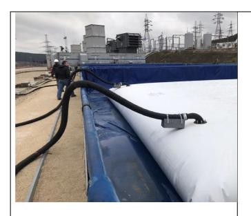
Polymer elastic tanks are intended for storage and transportation of jet fuel, aviation kerosene, diesel fuel, gasoline, engine oils and crude oil in field conditions, at ambient temperatures from minus 60 ° C to plus 80 ° C. Height of Polymer elastic tanks is 1,70
